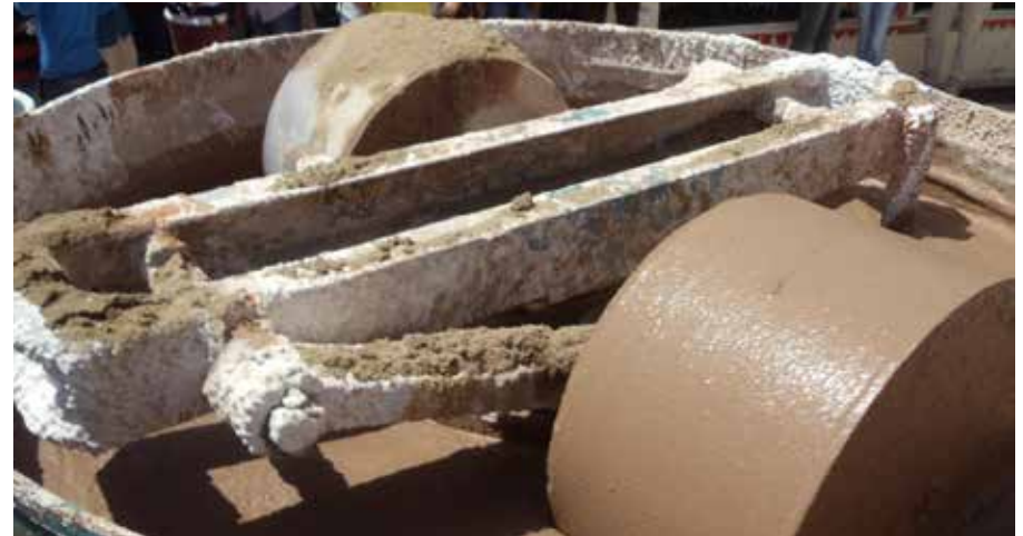
Fig 60: Image showing mixing of lime in mechanical Gharat
